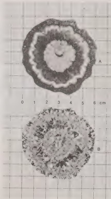
Figure 13: Section through the centre of a large hailstone. (A) Alternate layers of opaque (white) and transparent (black) ice seen in reflected light. (B) The individual crystals seen in polarized light. The opaque layers are composed of small crystals and the transparent layers of much larger crystals.
